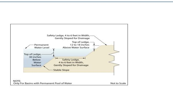
E. Safety Ledge Illustration Elevation View – Basin Safety Ledge Configuration
